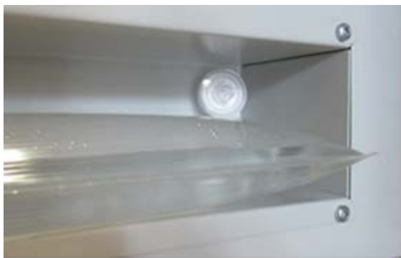
Figure 53: Location of the gas fine filter (sterile filter) in the recess for the freshwater bag
