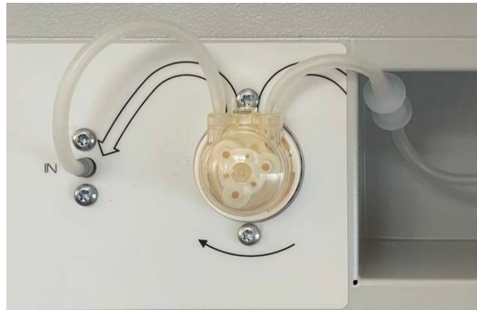
Figure 21: Water supply via freshwater bag, assembled
